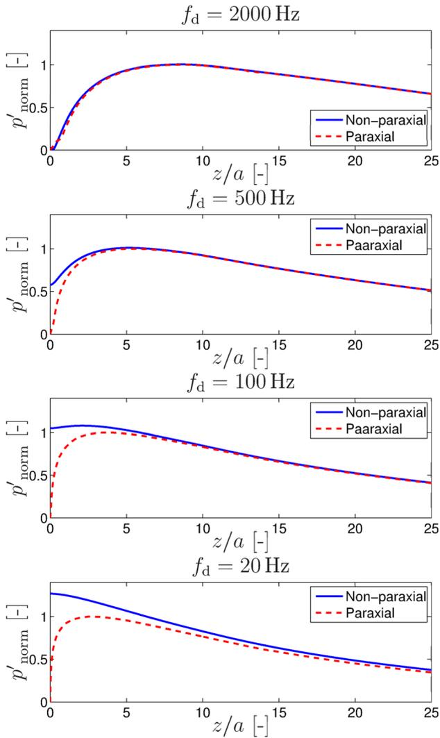
FIG. 3. (Color online) Distribution of normalized acoustic pressure amplitude of the difference-frequency wave along the piston axis for different values of  $f_d$ . In the non-paraxial approximation, integral (10) was used, in the paraxial approximation, integral (11) was used.
