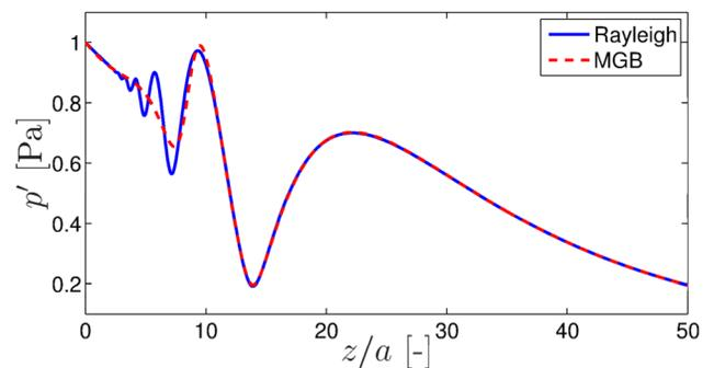
FIG. 2. (Color online) Distribution of the primary wave acoustic pressure amplitude along the piston axis calculated using Eq. (8) and the Rayleigh integral (4),  $f_a = 50$  kHz,  $v_{0a} = 2.43 \times 10^{-3}$  m · s<sup>-1</sup>.
